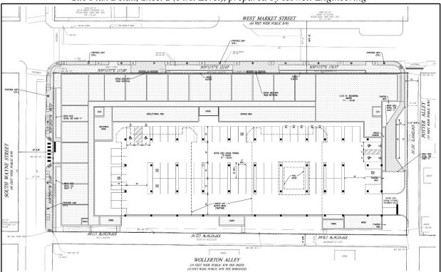
Site Plan Detail, Sheet 3 (Second Level), prepared by Howell Engineering
