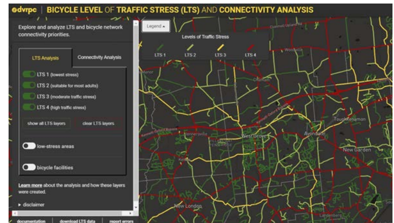
DVRPC Level of Traffic Stress. This tool was utilized to evaluate the level of stress bicyclists would experience where split-mode facilities were deemed necessary due to physical constraints or private property concerns.
